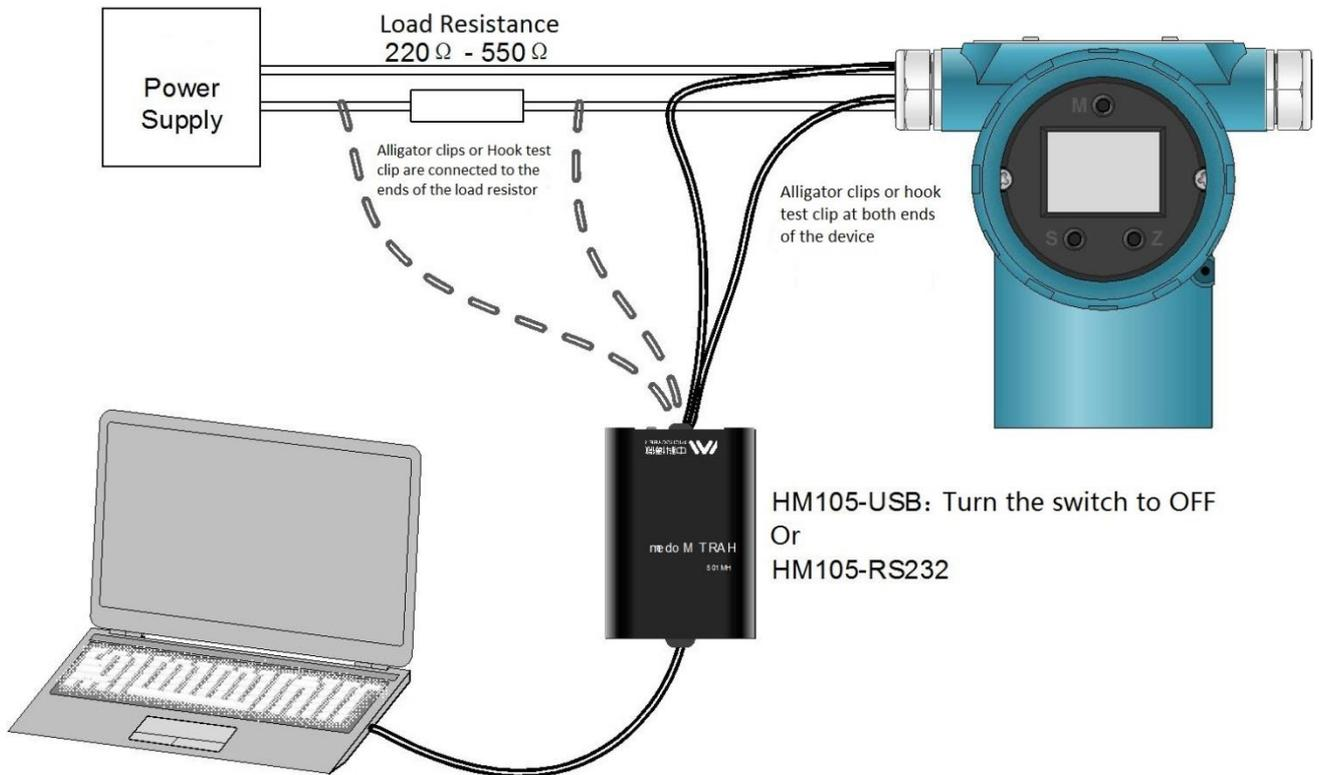
Figure 4 HM105-USB (OFF) or HM105-RS232 Wiring diagram
