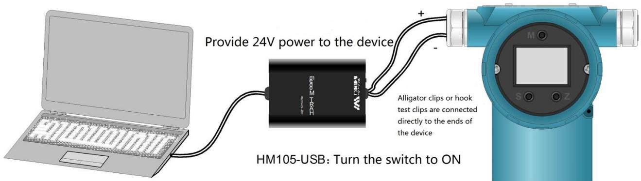
Figure 5 HM105-USB (ON) Wiring diagram
